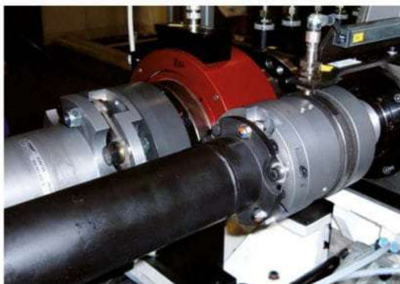
ROBA®-DS shaft coupling combined with an EAS®-torque limiter in a gear test stand manufactured by the company EGM (Entwicklungsgesellschaft für Montagetechnik GmbH).
