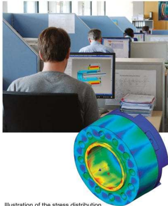
Illustration of the stress distribution in a backlash-free shaft connection
